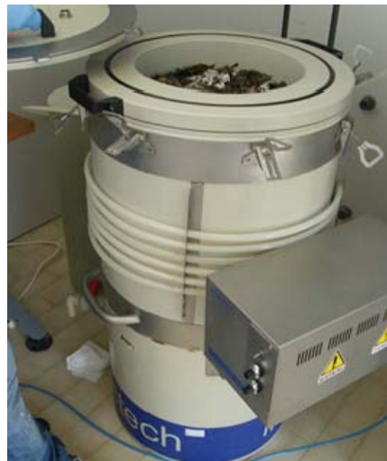
Figura 6.18 Respirometro adiabatico Costech International
