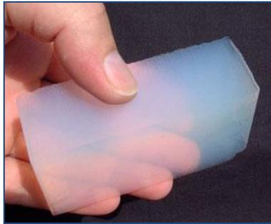
**Figure 1.** Silica aerogel
