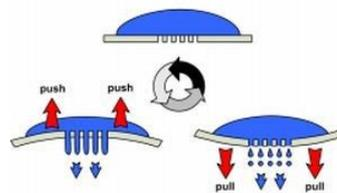
**Figure 8:** Working principle of the vibrating mesh
