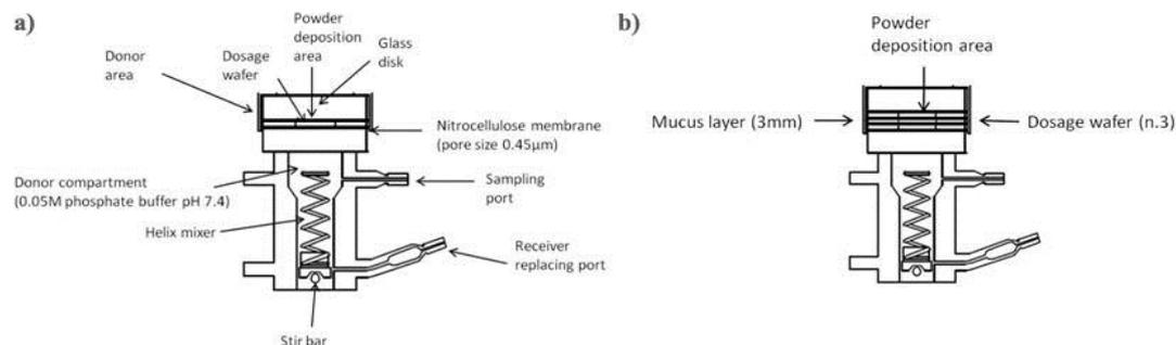
**Figure: 47.** Franz cell used in permeation studies: a) standard configuration with one dosage wafer housing the drug formulation; b) modified configuration with three dosage wafers housing mucus and drug formulation.
