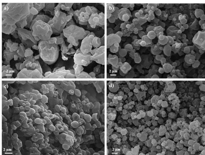
**Figure 20:** SEM pictures of powders obtained from a) #2 (110°C, 3% w/v, 7 $\mu\text{m}$  nozzle), b) #1 (110°C, 5% w/v, 7 $\mu\text{m}$  nozzle), c) #4 (110°C, 3% w/v, 4 $\mu\text{m}$  nozzle), d) #3 (110°C, 5% w/v, 4 $\mu\text{m}$  nozzle).
