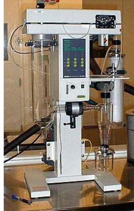
**Figure 5:** Mini Spray Dryer
