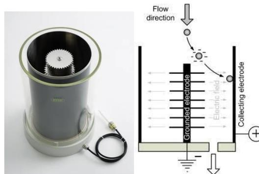
**Figure 9:** Electrostatic particle collector
