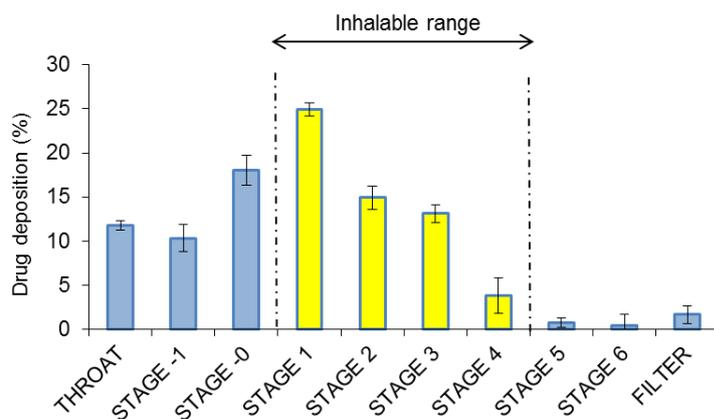
**Figure 21:** Andersen cascade impactor deposition pattern after the aerosolization of powder (batch #5) sprayed with a 4  $\mu\text{m}$  nozzle at 70°C (#5% N4T70).
