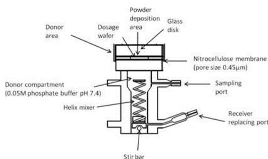
**Figure 25:** Franz cell used in permeation studies: a) standard configuration with one dosage wafer housing the drug formulation; b) modified configuration with three dosage wafers housing mucus and drug formulation.
