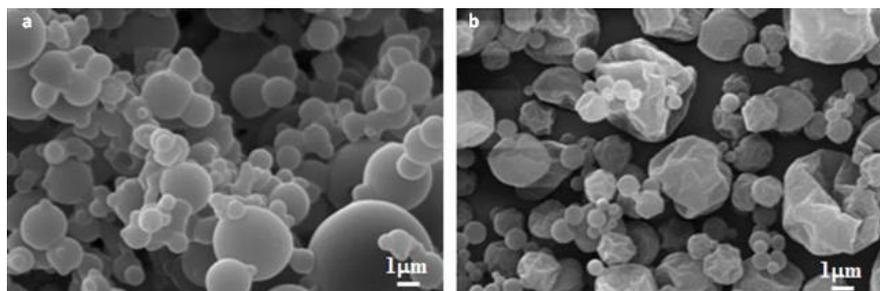
**Figure 17:** SEM pictures of spray-dried powders: a) Klys-1a batch containing API alone, and b) Klys-2a batch containing API and leucine as an additive.
