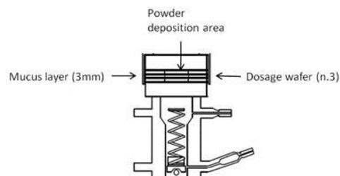
**Figure 28:** Modified configuration of Franz cell used in permeation studies with three dosage wafers housing mucus and drug formulation.
