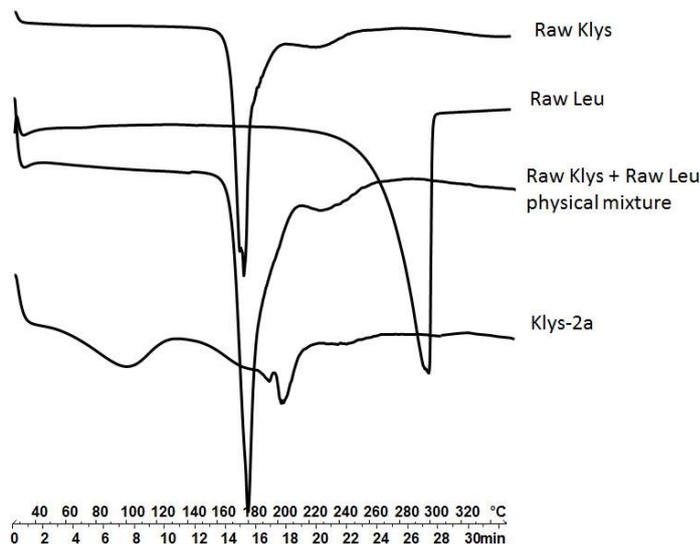
**Figure 18:** Differential scanning calorimetry thermograms of ketoprofen lysinate and leucine raw materials, of their physical mixture and of the spray-dried powder Klys-2a.
