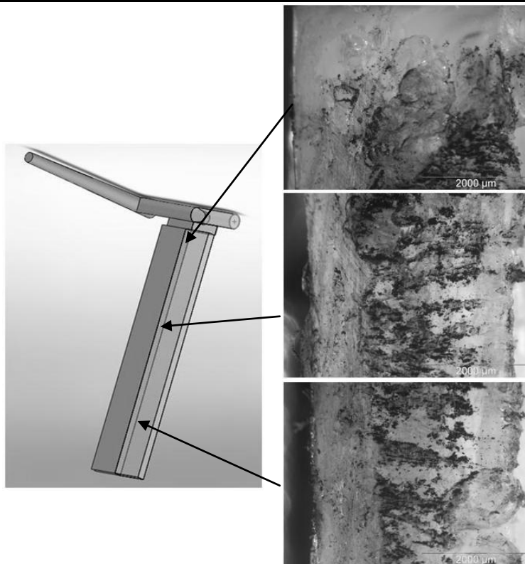
Figure 126. Micrographs of the foamed samples of PLA 4032D molded with back pressure 2 bar ( T=200^{\circ}\text{C} ).
