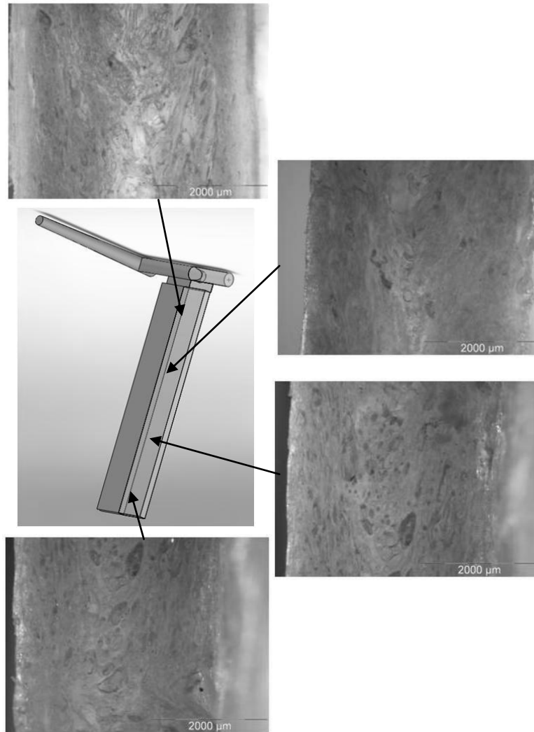
Figure 129. Micrographs of the foamed samples of PLA 4032D molded with back pressure 3 bar ( T=200^{\circ}\text{C} ).
