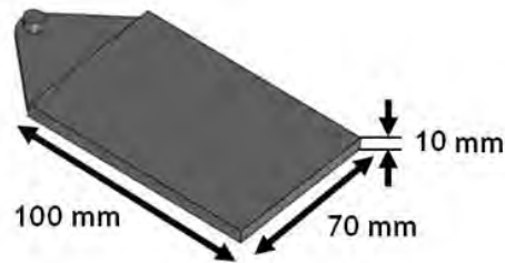
Figure 55. Samples geometry utilized in the first set of experiments with PS 678E.
