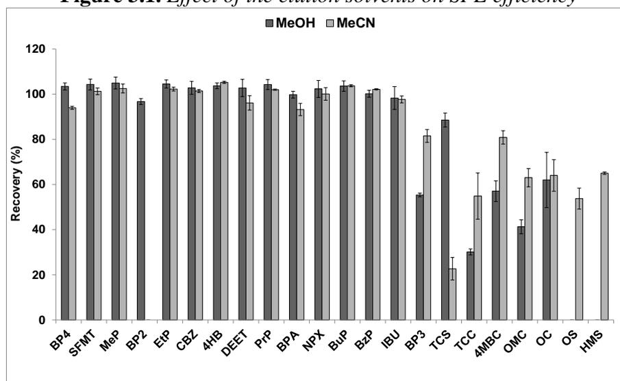
Experimental conditions: HLB, 200 mg, volume of elution solvent, 3 x 3 mL (n = 3).
