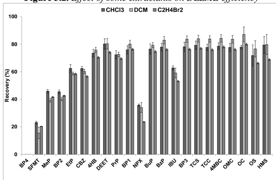
Experimental conditions: water volume, 5 mL; disperser solvent, MeCN 800  $\mu\text{L}$ ; Volume extraction solvent, 200  $\mu\text{L}$  (n= 3).
