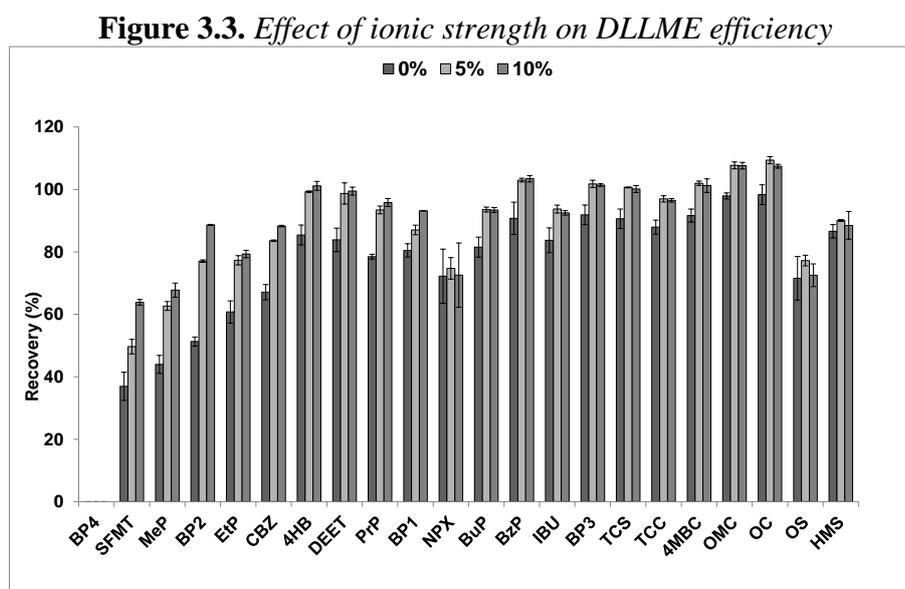
Experimental conditions: water volume, 5 mL; disperser solvent, MeCN 800  $\mu$ L; Volume extraction solvent, 200  $\mu$ L (n= 3).
