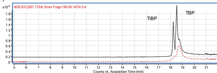
Such a disturbance was observed even for simulated injections of empty vessels (Figure 4.1), and it was noticed with different LC columns. Replacement of ACN by methanol and formic acid by ammonium acetate as organic mobile phase and modifier, respectively, did not overcome the problem. Thus, the origin of TBP contamination was attributed to ultrapure
