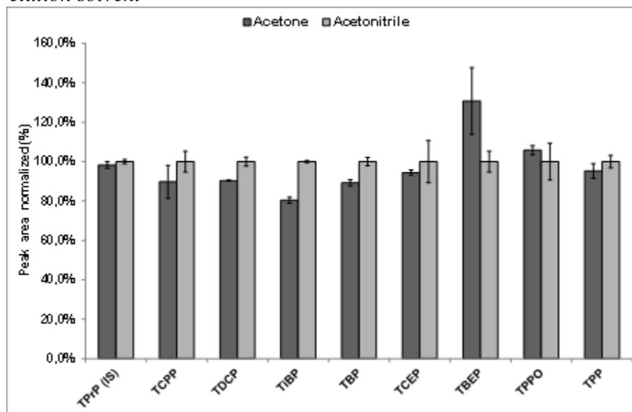
Experimental conditions: sludge, 0.5g; spiked level, 1000 ng mL<sup>-1</sup>; Dispersant sorbent, 2 g diatomaceous earth; elution solvent volume, 15 mL; n = 4.
