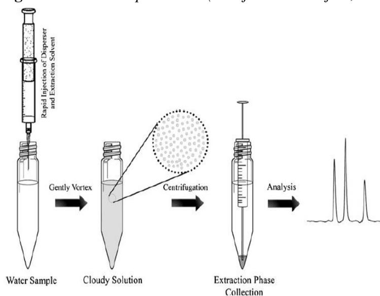
The performance of DLLME is assessed in terms of two different parameters, namely, the enrichment factor (EF) and the extraction recovery (ER). EF is defined as the ratio of the analyte concentration in the sedimented phase ( $C_{sed}$ ) to its initial concentration in the aqueous sample ( $C_0$ ) (Rezaee *et al.*, 2006):
