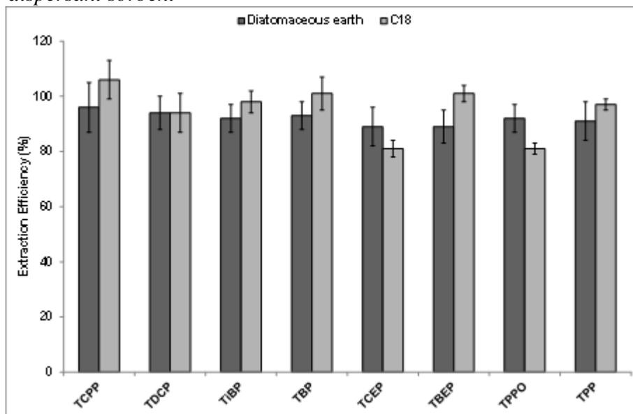
Experimental conditions: sludge, 0.5g; spiked level, 1000 ng mL<sup>-1</sup>; Dispersant sorbent, 2 g; eluent solvent, 15 mLacetonitrile; n = 4.
