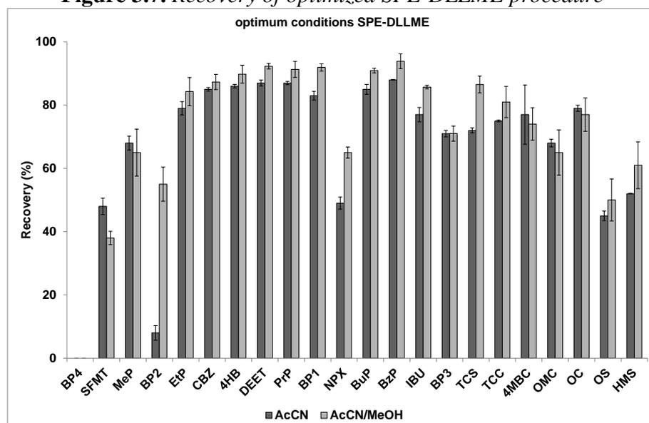
Experimental conditions: SPE eluent, 5 mL MeCN/DCM 6:4, v/v or MeCN/MeOH/DCM 3:3:4, v/v/v; DLLME mixture extractant/dispersant, 2 mL SPE eluate; aqueous phase 10 mL 5% w/v NaCl; final extract volume DLLME, 200  $\mu$ L (n = 6).
