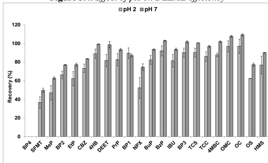
Experimental conditions: aqueous phase NaCl 5% (w/v), 5 mL; disperser solvent, MeCN 800  $\mu$ L; Volume extraction solvent, 200  $\mu$ L (n= 3).
