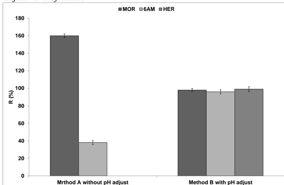
SPE extraction efficiency evaluated adding ISs after SPE.
