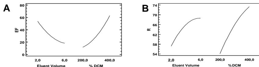
The eluent volume (A) negatively affected EF (EF decreased with the enhancement of A) (Figure 3.6A) due to dilution of the analytes in the SPE eluate and consequently in the aliquot subjected to DLLME. On the other hand, DCM percentage (B) had a positive effect on EF (Figure 3.6A), because a greater DCM percentage increases the eluotropic strength of SPE eluent reducing consequently its volume.
