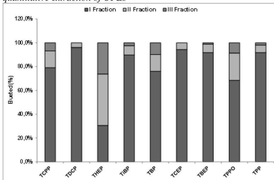
Experimental conditions: sludge, 0.5g; spiked level, 1000 ng mL<sup>-1</sup>; Dispersant sorbent, 2 g C18; eluent solvent, acetonitrile 5 mL (x3); n = 4.
