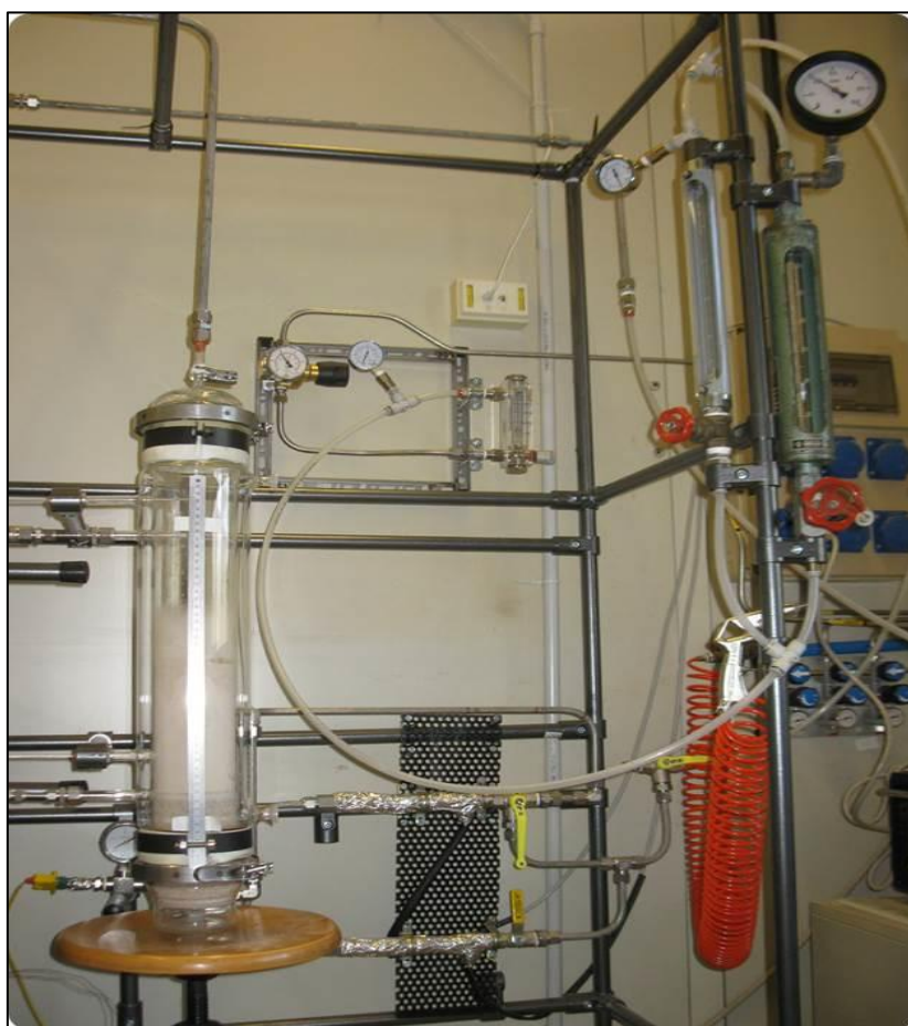
Figure II.3. Picture of the lab-scale batch fluidized bed torrefier.
