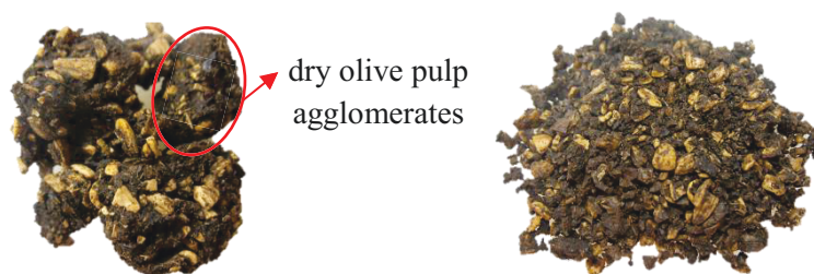
Figure II.5 Picture of (left) air-dried virgin olive husk and (right) air-dried olive husk further processed by using a knife mill.
