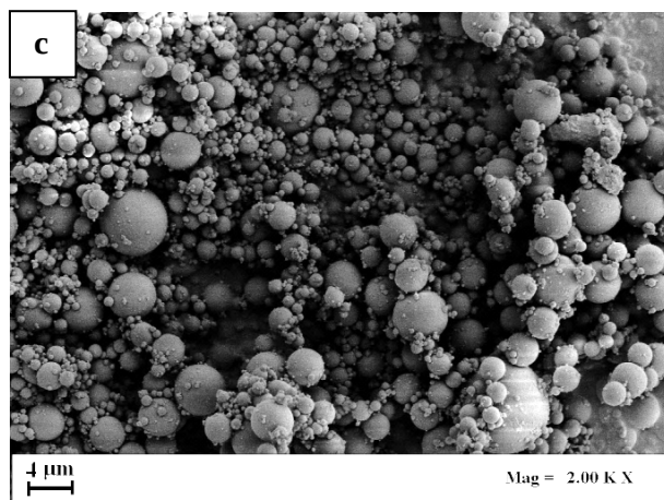
Figure VI.15 FESEM images of lysozyme microparticles obtained using an Isopropyl alcohol flow rate of: (a) 10 mL/min; (b) 15 mL/min; (c) 25 mL/min.
