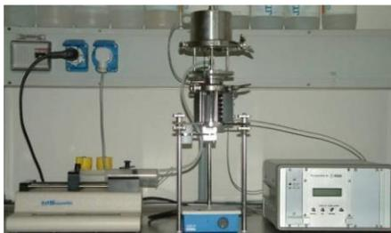
**Figure 5.** Vibrating nozzle device Nisco Encapsulator Unit, Var D.
