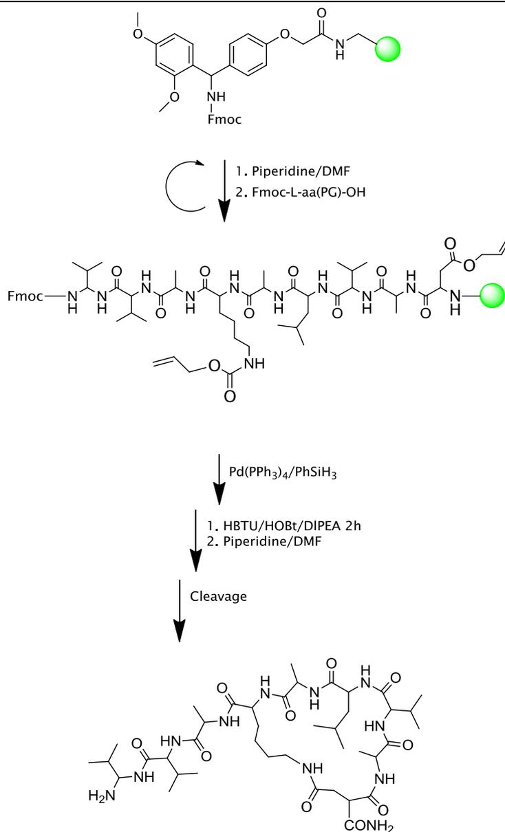
**Figure 3.11** Schematic representation of the lactam cyclic peptide synthesis.
