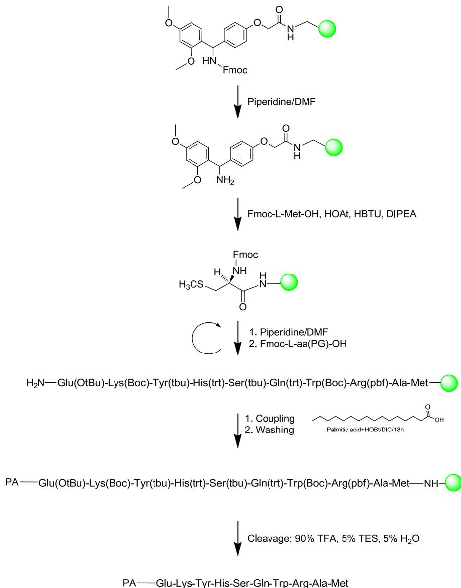
**Figure 4.2.** Schematic representation of the peptide **PA-5** synthesis.
