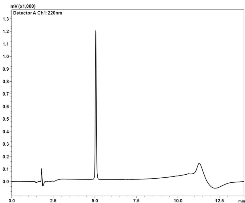
**Figure 3.12** Analytical HPLC spectrum of peptide 25.
