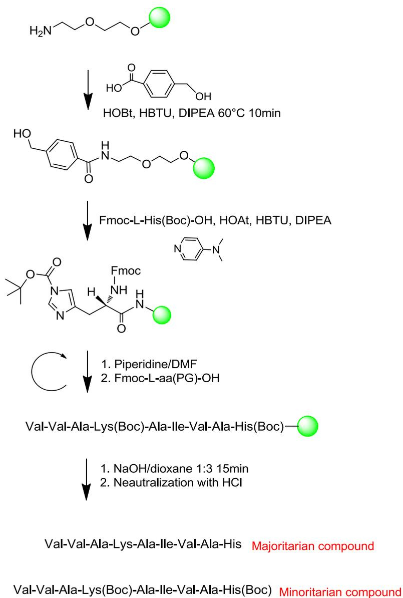
**Figure 3.9** Schematic representation of the cyclic peptide synthesis.
