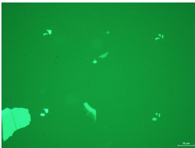
Figure 20. A grid referenced-markers The distance is 75um along x and 40um along y .
