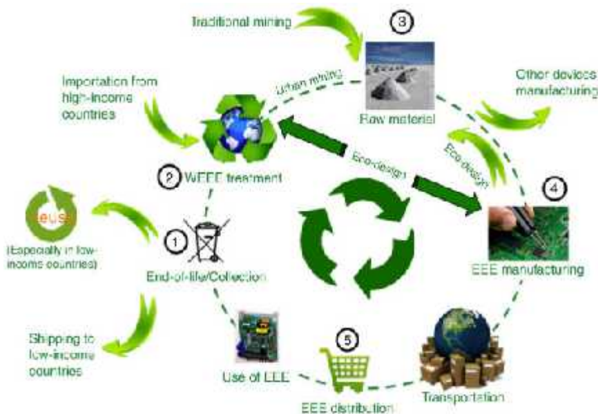
Figure 2.1 Theoretical circular economy scheme for WEEE management: (1) WEEE collection; (2) WEEE treatment; (3) Return of recovered materials into the market; (4) manufacturing of new EEE; (5) commercialization of new EEE (Chagnes et al., 2016).
