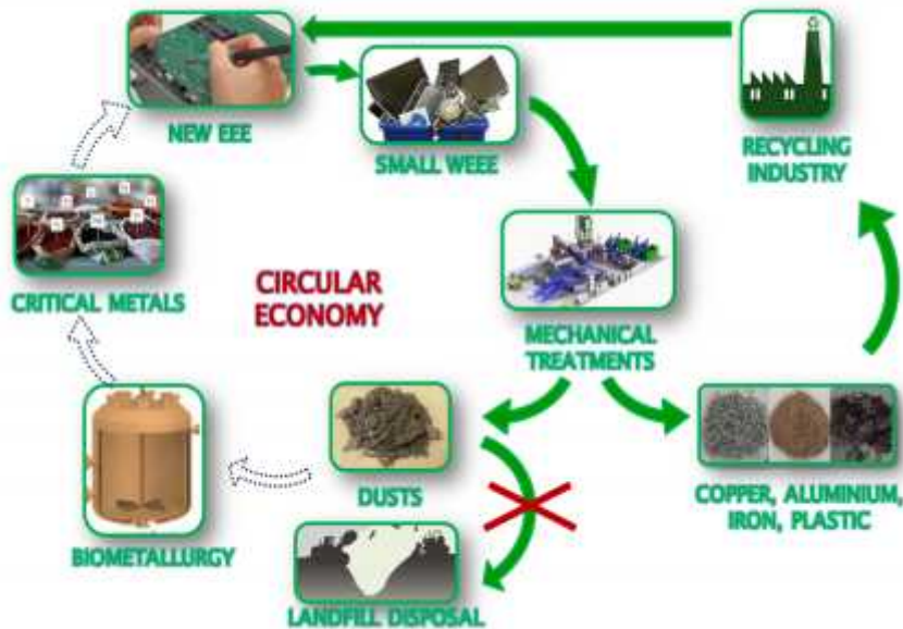
Figure 7.16 A circular economy approach for the management of dust coming from WEEE mechanical treatments
