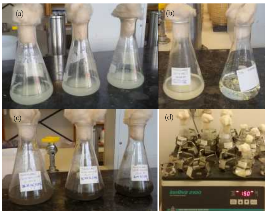
Figure 6.7 Bioleaching medium containing active growing cultures of A. thiooxidans (a), inoculated and non-inoculated bioleaching medium (b), bioleaching medium containing active cultures and dust material at different pulp density (c), bioleaching experiments (d)
