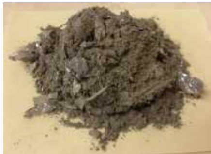
Figure 6.4 Dust material used for hydro-biometallurgical tests
