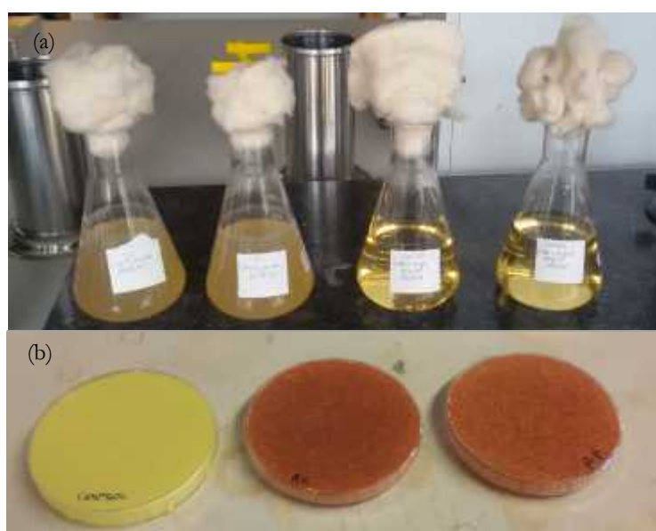
Figure 6.8. Inoculated bioleaching medium containing active growing cultures of P. putida and non-inoculated flasks (a), colour reaction proving the \text{CN}^- production of P. putida (b)
