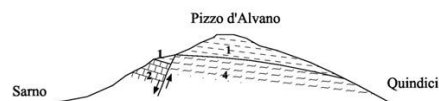
Figure 8.2 Geological map of Pizzo D'Alvano massif: 1) calcarenites and calcirudites (Upper Cretaceous), 2) calcarenites, calcilutites and dolomitized limestone (Middle-Upper Cretaceous), 3) marly limestone (Middle Cretaceous), 4) microcrystalline limestone partially dolomitized (Lower-Middle Cretaceous), 5) dolomitized limestone (Lower Cretaceous) (Cascini et al., 2008).
