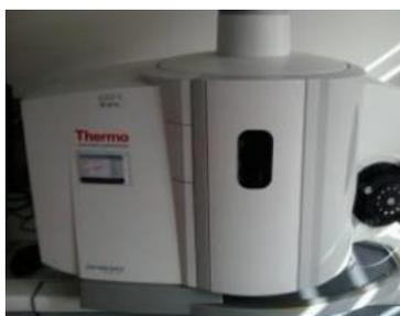
*Figure 6.14 ICP-OES (Thermo electron corporation-Icap6000 series)*
