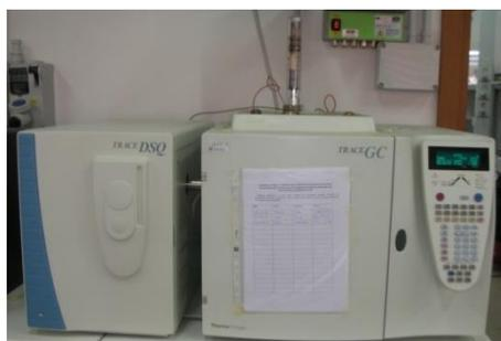
Figure 6.12 GC-MS (ThermoFinnigan DSQ Trace)
