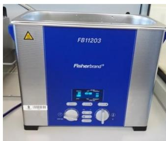
Figure 6.21 Ultrasonic bath (Fisherbrand model FB11203)
