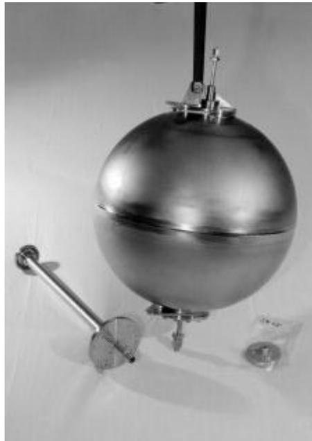
**Figure 2.20 – Attitude Control System (SCA) tank of welded Ti-6Al-4V SPF half shells**
