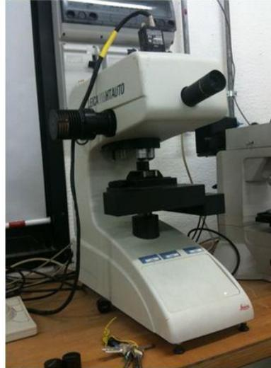
**Figure 4.13 – LeicaVM HTAUTO micro hardness tester**
