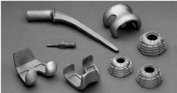
**Figure 2.23 – Components of a hip implant made from cast titanium**
