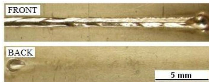
Figure 4.17 – BoP at 1400 W, 110 mm/s and -2 mm
