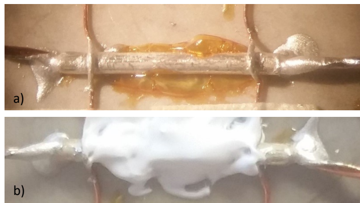
Fig. 2.12: Bi-2212 sample coupling with the sample holder by means of G-Varnish (a), and thermal conductive gel (b)
