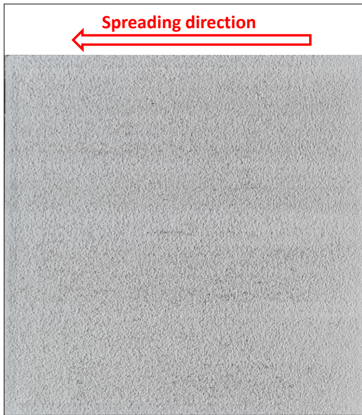
Figure V.6 Macroscopic image of the deposited powder layer for V_s equal to 3 \cdot 10^{-2} \text{ m s}^{-1} when the powder has been re-used.
