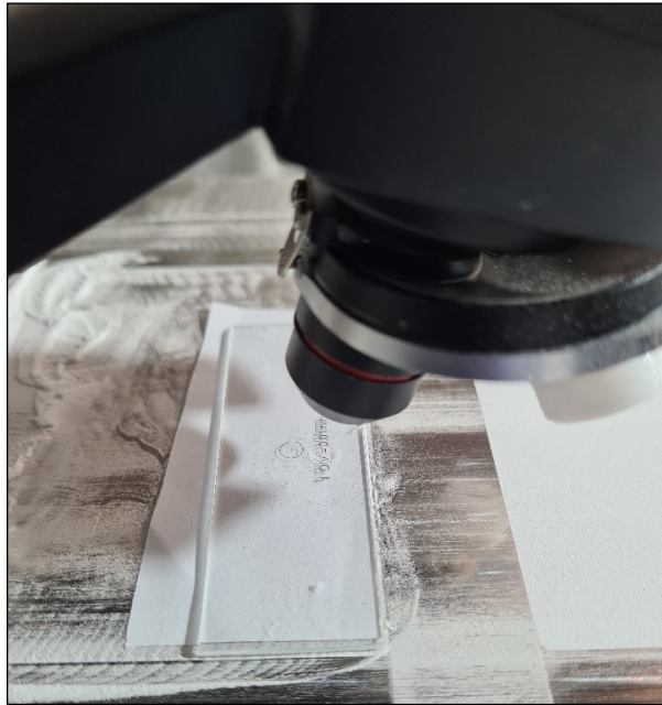
Figure III.19 Calibration procedure based on the measure of the distance between two tick marks on the microscope slide by using the microscope coupled with the camera.
