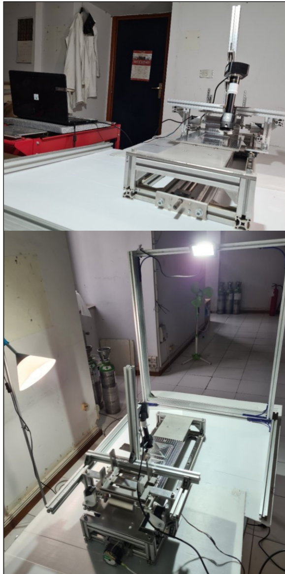
Figure III.14 Some views of the setup with the connection for the microscope and proper lightning for the image analysis of the powder layer.
