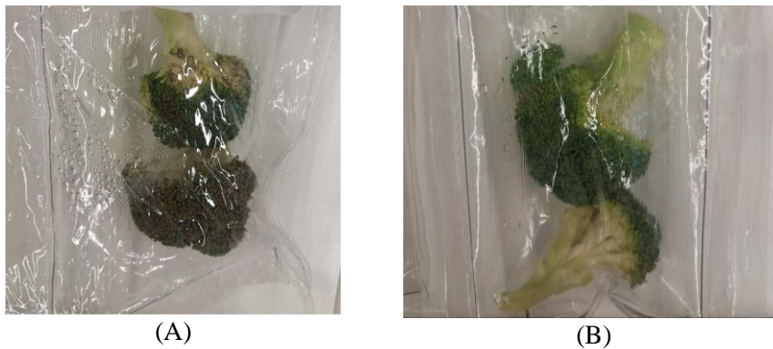
Figure 17 Broccoli florets packaged in neat PET film (I, left) and in active monolayer film (A, right) taken as example, after 1 day of storage at 5°C.
