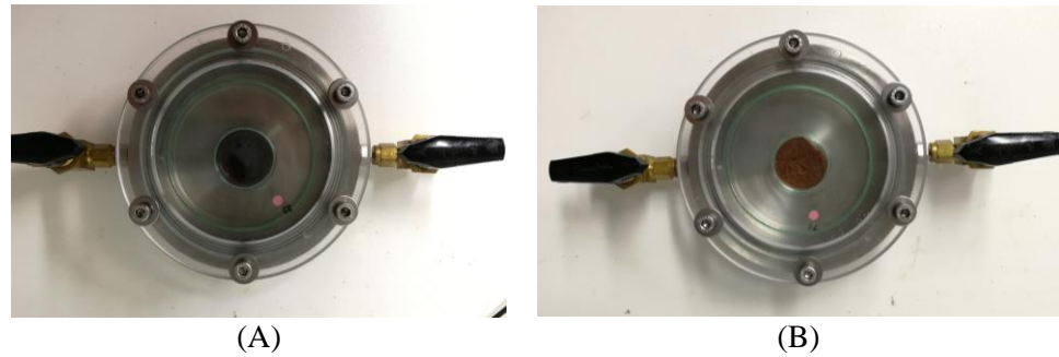
Figure 43 Experimental setup for oxygen absorption measurements of OPE_liq (A) and OPE_powder (B).
