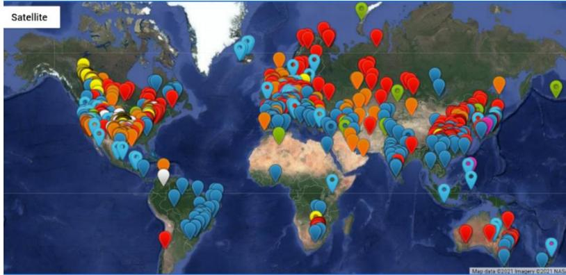
**Figure 1.4** - World map showing 1229 projects with reported induced seismicity. Source: The Human-Induced Earthquake Database (HiQuake - <https://inducedearthquakes.org/>, last accessed March 2021)
