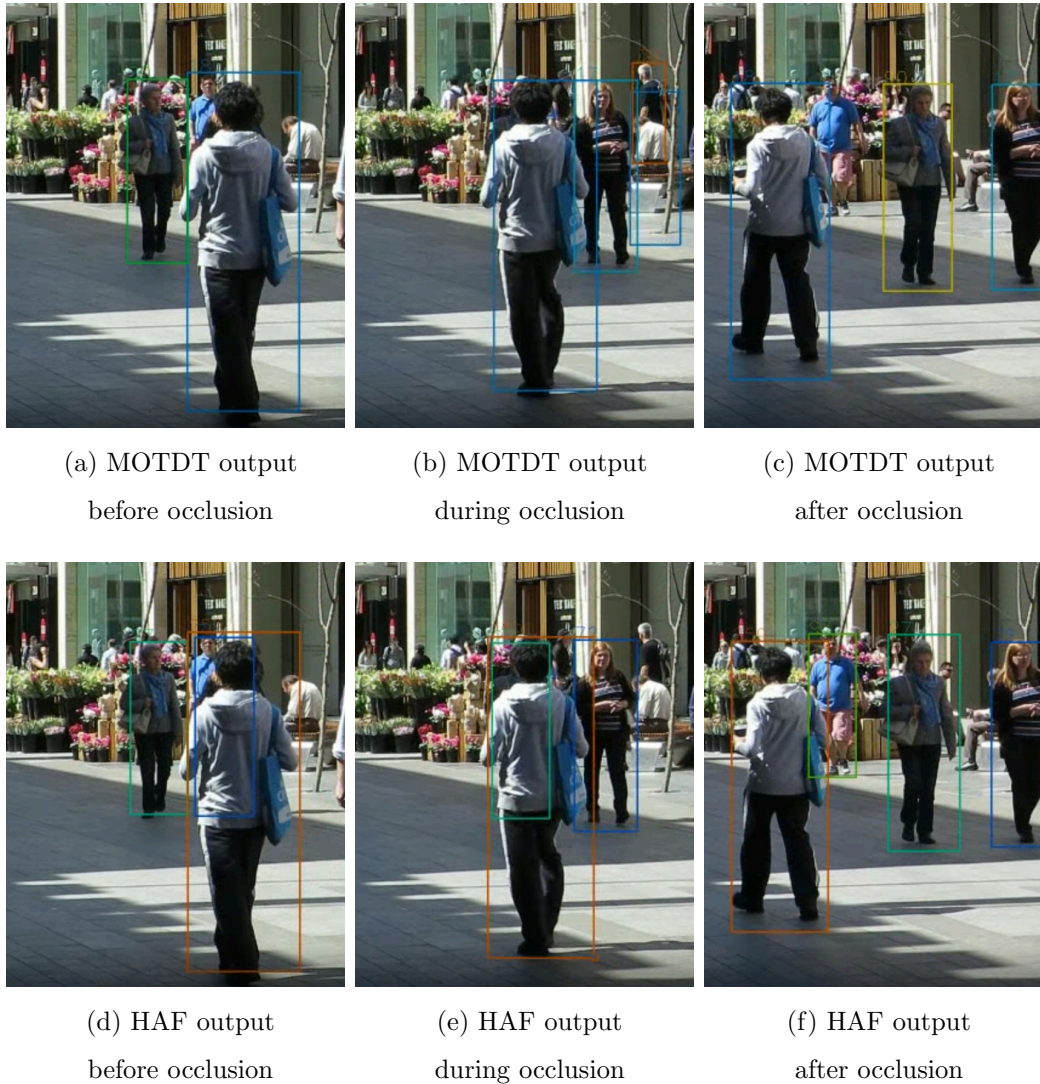
Figure 3.7: Example of fragmentation produced by an online method during occlusion. Above: tracking results for MOTDT [139], online algorithm. Below: tracking results for HAF [125], batch algorithm. From left to right, frames 145, 170 and 217 of the MOT17-08 video are shown. Images were cropped from the public MOTChallenge website and show results using the public detections. The person in 3.7a surrounded by the green box is occluded in 3.7b by the one identified by the blue box. The tracking is lost (fragmentation) until the occlusion ends in 3.7c (the person is also given a new ID, causing an ID switch). In contrast, we can see how in 3.7e the track is maintained through the occlusion, since the batch algorithm can look at the future information (e.g. frame 3.7f) and infer the position of the target during occlusions.
