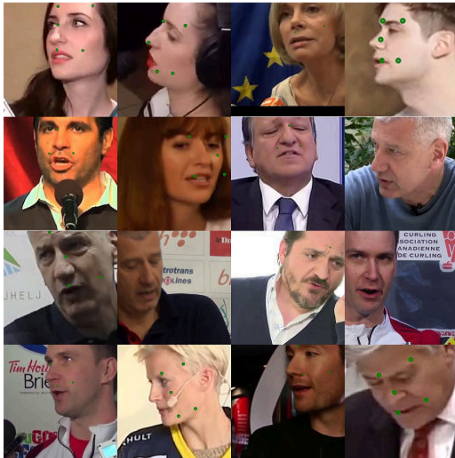
Figure 4.17: 16 examples of landmark prediction failures by MTCNN that resulted in low AP for ArcFace with ResNet-101 (configuration 37). Images have been resized to be 256 pixels wide. Zoom in to see the green circles representing the five facial landmarks (eyes, nose tip, mouth corners) predicted by MTCNN. Some faces have less than five landmarks because the predicted coordinates for some of them were outside of the image boundaries.
