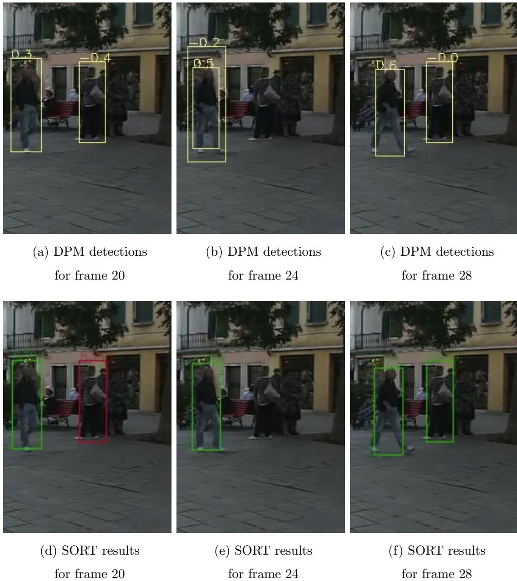
Figure 3.8: Influence of detection failures on the SORT algorithm. The images show frames 20, 24 and 28 of the MOT17-01 video. Images were cropped from the public MOTChallenge website. Above: public DPM detections provided with MOT17. Below: tracking results using SORT [61], when applied to the DPM detections. We can see how as soon as the central target is not detected in 3.8b, SORT loses the target too (3.8e). When the detector finds it again (3.8c), tracking is restored (3.8f), but with a different ID (since SORT does not perform person re-identification).
