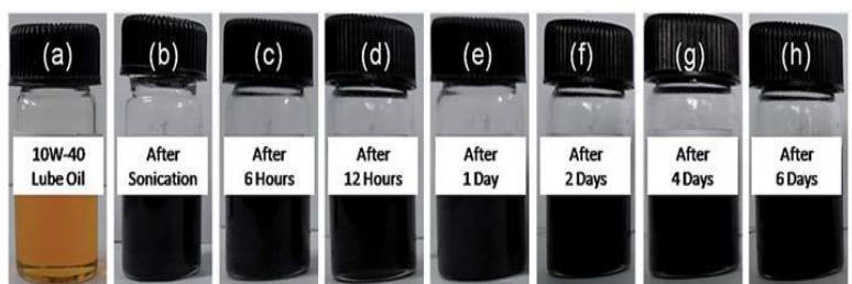
Figure 4.5 Photos of (a) 10W-40 lube oil and (b–k) dispersions of GO–ODA nanosheets in 10W-40 lube oil at different times (up to one month). Time is reported on each bottle. Concentration of GO–ODA nanosheets: 0.04 \text{ mg mL}^{-1} (Mungse, Kumar and Khatri, 2015c).
