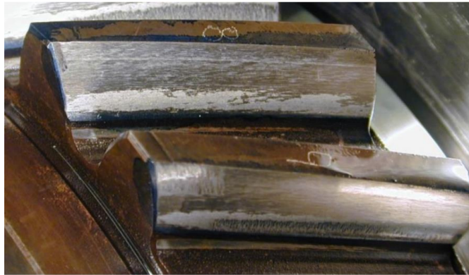
Figure 2.5 Gear micropitting (grey staining) exposure to contact fatigue (Sun, Giusca and Lancaster, 2017).
