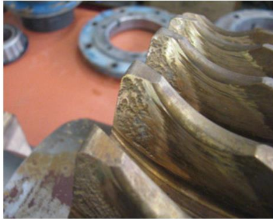
Figure 2.2 EP additives are causing damage to a bronze worm wheel (Cash, 2012).
