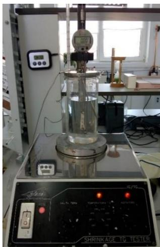
Figure 39. The shrinkage tester
