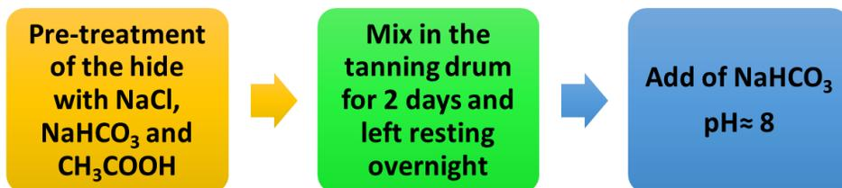
Figure 81. Scheme of the lab-scale wet-white tanning process.
