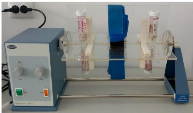
*Figure 30. Rotator drive stirrer STR4 used for simulating the tanning drum.*
