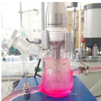
Figure 76. Sonic vibracell VCX 750 with a 13mm probe in titanium.
