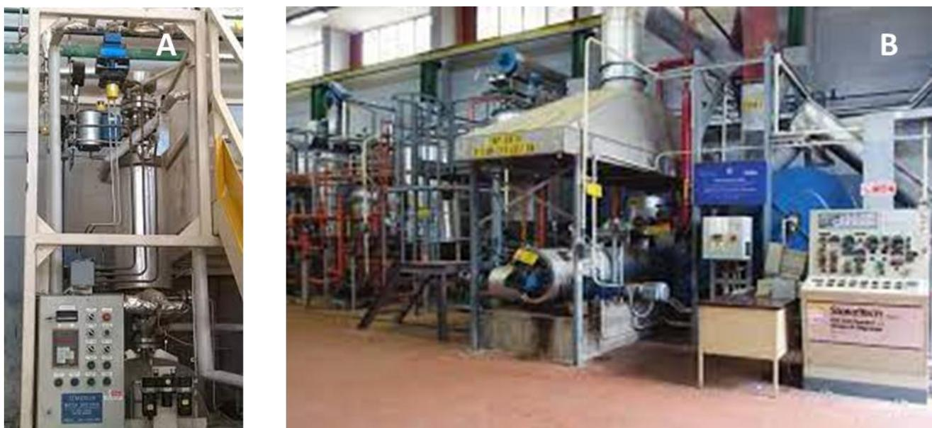
**Figure 33.** Steam explosion technology in ENEA (Trisaia): batch plant (A) and continuous plant (B)
