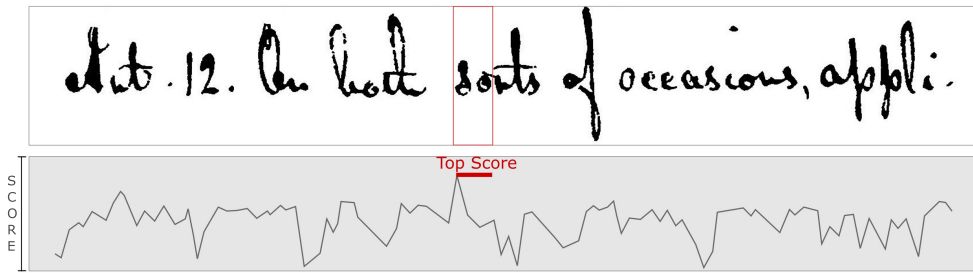
Figure 5.8: The sliding window cuts out the image portions of a line of text and the similarity score calculated with the reference N-gram is reported for the entire line. The score trend helps identify where the reference N-gram might be.
