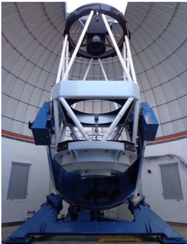
Figure 2.5: The 1.6 m telescope located in South Africa for the KMTNet collaboration. Credit image: KMTNet collaboration
