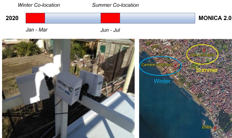
Figure 2.3 Field calibration scheme with a Google Earth view of the co-location and a photo of 4 MONICA 2.0 mounted on the roof of the mobile laboratory.
