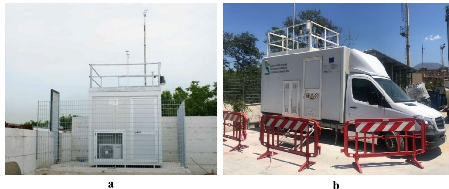
Figure I. 2 Typical fixed-site air quality monitoring station a); Mobile air quality monitoring station b).
