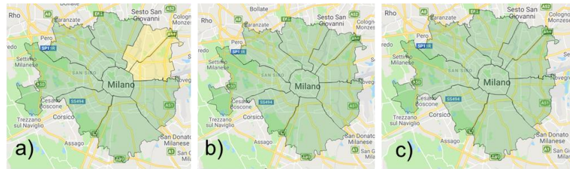
Figure III.6.1. Map of a) PM2.5 mean concentration, b) PM10 mean concentration, c) NO 2 mean concentration divided by districts. Color codes are provided in Table 12. Red represents pollutant concentrations above the air quality limits, yellow indicates an almost good air quality and green indicates a good air quality. Grey represents the absence of data.
