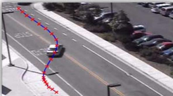
**Figure 2.3** A vehicle with anomalous trajectory.
